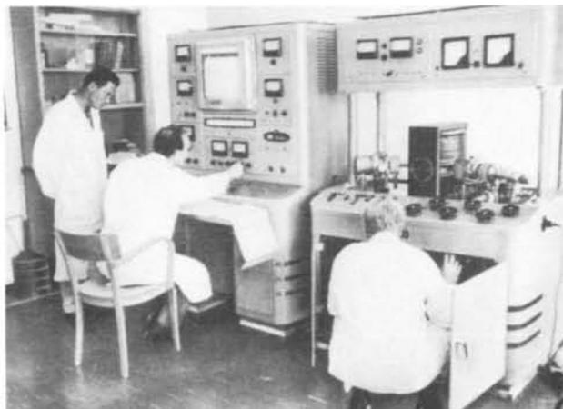
The mass spectrometer in the Seibersdorf laboratory being used to determine the nitrogen-15 content of some plant materials fed with fertilizer enriched in this stable isotope
