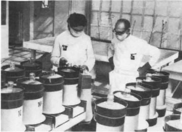
An IAEA technical assistance expert, Dr. Helge Bergh, of Norway, guiding work at the agricultural isotope laboratory set up with his assistance at the University of Ankara, Turkey. In the greenhouse of the laboratory, superphosphate labelled with phosphorus-32 is ready for mixing in with soils
