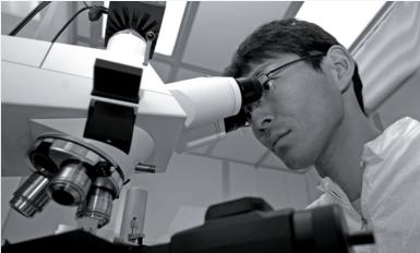
A technician at the Safeguards Analytical Laboratory in Seibersdorf examining uranium particles under an optical microscope. (Photo: D. Calma/IAEA)
