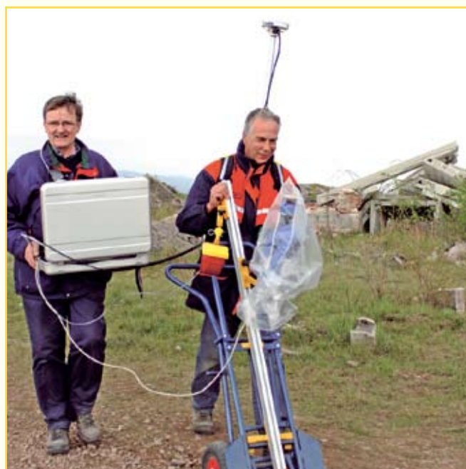
In Task 2, unknown gamma sources had to be localized, quantified and identified through a 'drive-by' reading.
