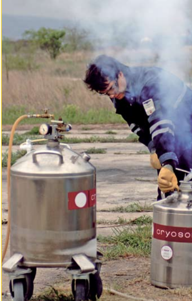
Liquid nitrogen is normally used to cool down the crystals in the spectrometers. A container with the cooling element was available on site for the teams to refill their tanks.
