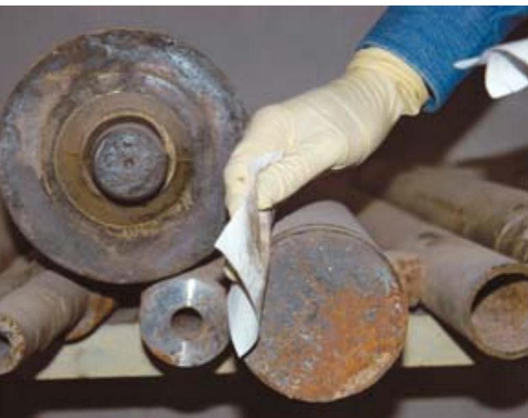
Safeguards activities include the collection of environmental samples analyzed at the IAEA Safeguards Analytical Laboratory and network laboratories worldwide. (Credit: Pavlicek/IAEA)
