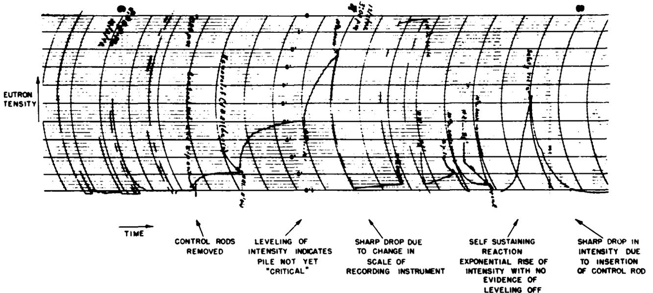
Photocopy of the instrument chart used during the start-up of the Chicago pile. This chart is often referred to as the "birth certificate" of the atomic age (Photo Argonne National Laboratory)
