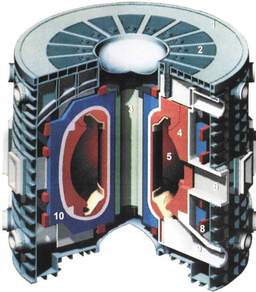
Computer-generated model of the International Thermonuclear Experimental Reactor (ITER), the fusion device that when built would be about 30 meters high. Shown are 1) the cryostat vacuum vessel; 2) vertical access port; 3) central solenoid; 4) blanket/shield; 5) plasma chamber; 6) port to provide access to plasma chamber; 7) divertor; 8) poloidal field magnet; 9) vacuum pump duct for exhaust; 10) toroidal field magnet.
