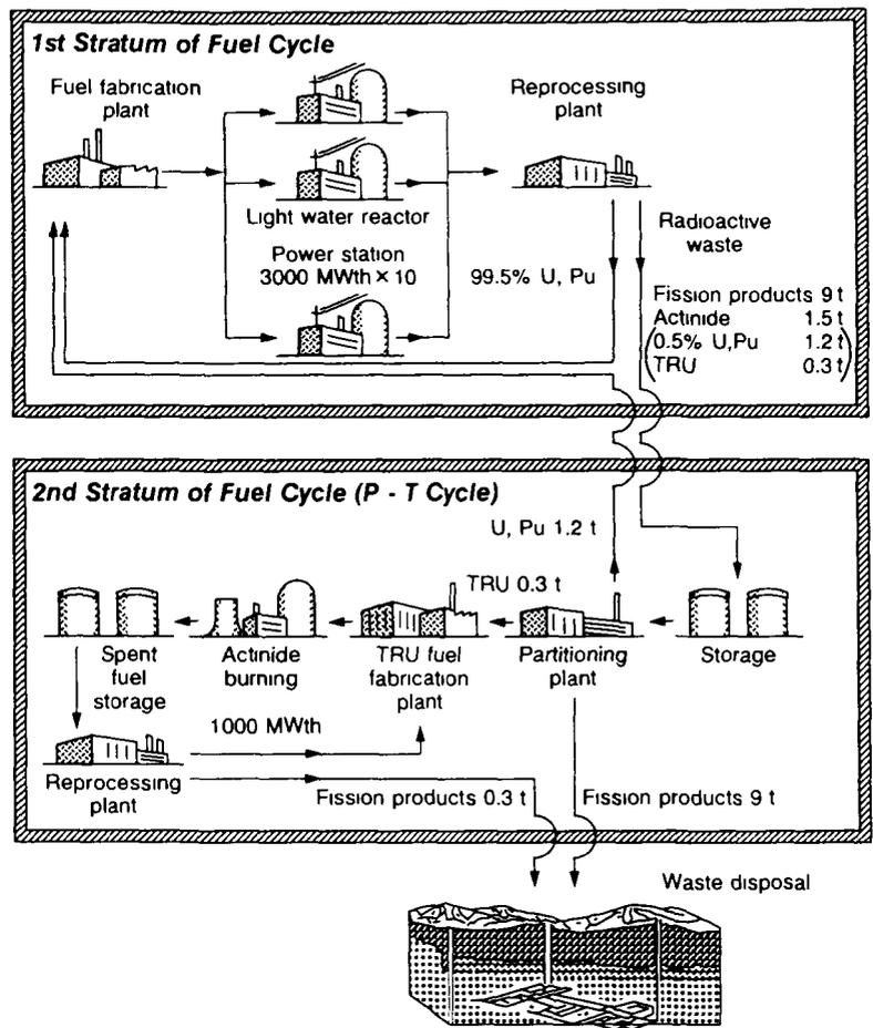
is that all actinide elements would be recovered, recycled, and consumed. Several universities have put forward concepts for using high-energy particle accelerators in transmuted actinides and fission products.
