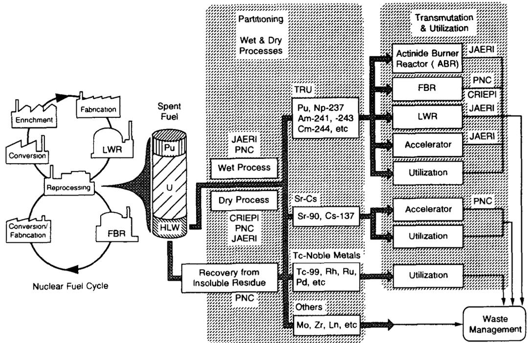
The fabrication technology of the separated TRU and fission products is to be developed for their further use or disposal. Immobilization of the separated strontium and caesium is needed for either their utilization or disposal.
