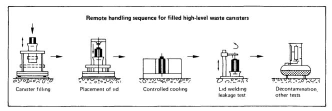
The figure shows the handling procedures for the glass canister generally implemented in vitrification plants based on both AVM and Pamela processes. After the glass is drained, the filled canister is subjected to a number of operations to prepare it for internal storage or ultimate disposal. The main operation steps are controlled cooling of the filled canister, welding of the lid, leakage testing, and decontamination.
