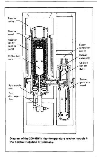
are due to the inherent properties of the coated particle fuel to withstand elevated temperatures without significant failure and the capability of the design concept to passively limit the temperature rise in the fuel during transients associated with postulated severe accidents.
