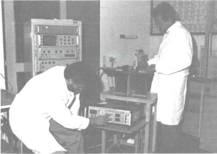
A microprocessor-based controller device used in density measurements of soil samples, designed by a trainee and constructed by the instrumentation unit of the PCI laboratory.
