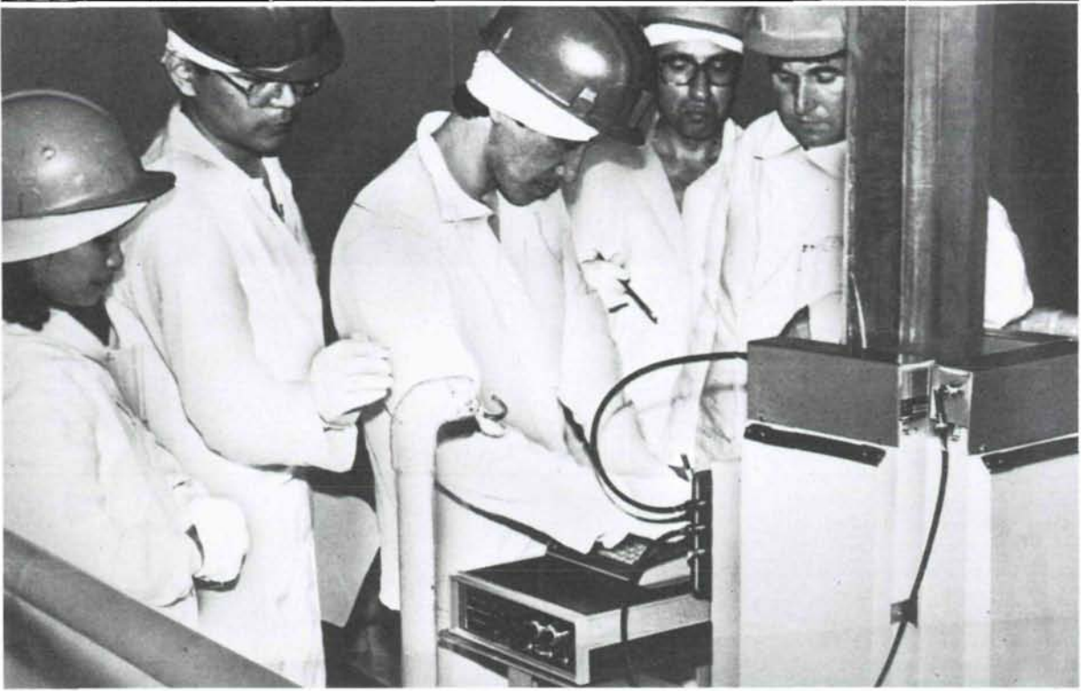
▲ During an inspection exercise in the USSR, IAEA staff and new inspectors measure the uranium content of a fresh VVER-400 fuel assembly using a uranium neutron coincidence collar. (Credit: USSR State Committee on the Utilization of Atomic Energy)
