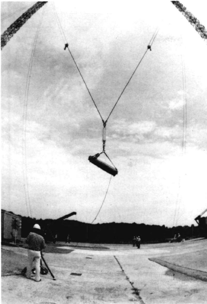
Crash, burn, and drop tests more demanding than actual transportation environments are among the torture trials spent-fuel casks have survived, with essentially no loss of containment and no significant reduction in shielding. (Credit: Atomic Industrial Forum, Inc.)
