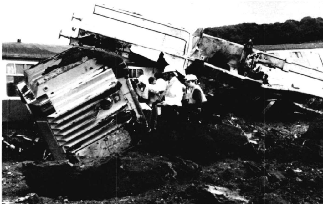
The patient survived: To further publicly demonstrate the structural integrity of shipping casks, the United Kingdom's Central Electricity Generating Board (CEGB) held a US $2.1 million test in July 1984 — a shipping cask was hit head-on by a diesel locomotive weighing 140 tonnes, coupled to three 35-tonne coaches and moving about 160 kilometres per hour. Despite the impact and being hurled 60 metres, the cask suffered only minor scratches and totally protected its contents, simulated nuclear waste, which were not affected. The train was demolished. (Credit: CEGB)
