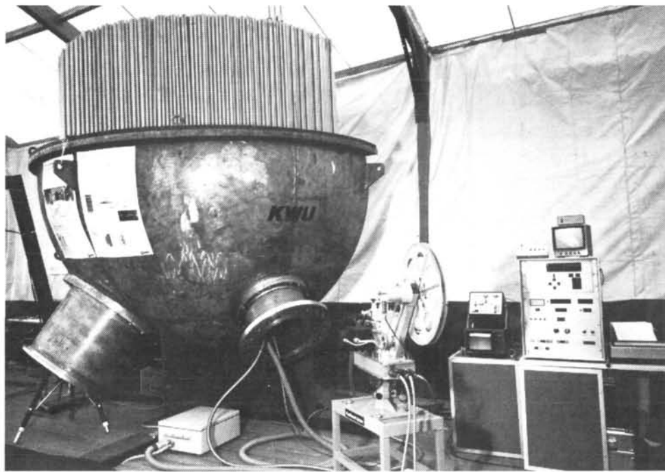
Figure 12. Primary chamber head mockup with eddy current equipment.
