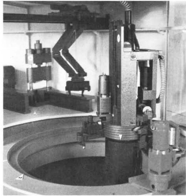
Figure 21. Top view of the heavy duty manipulator system showing the rotating ring girder opening.
