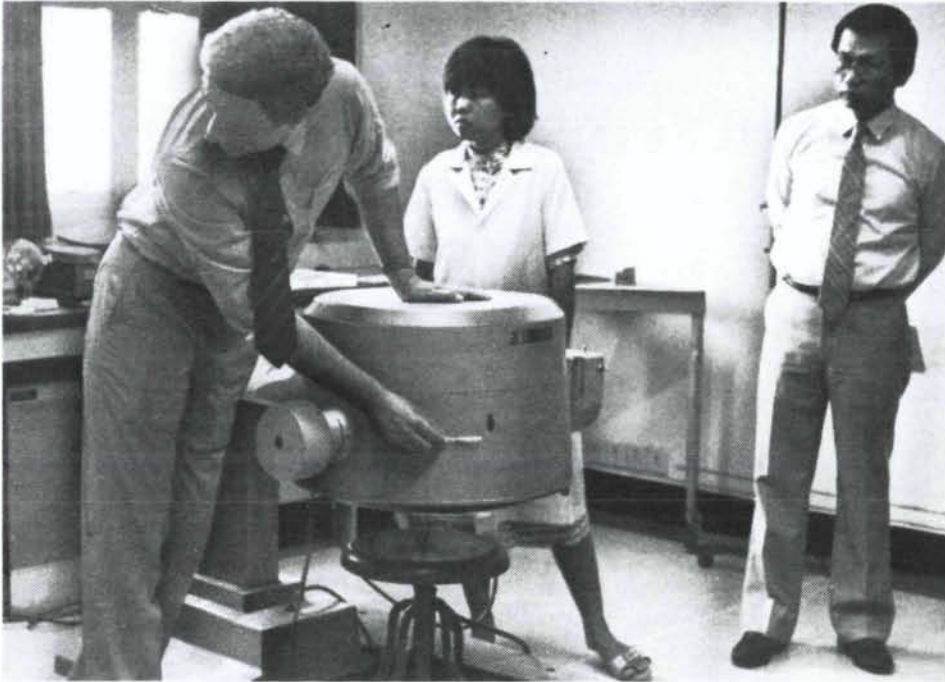
By using a small source of ^{99m}\text{Tc} , an Agency expert demonstrates leakage-testing of shielding of a gamma camera during a workshop at the seminar in Bangkok.
