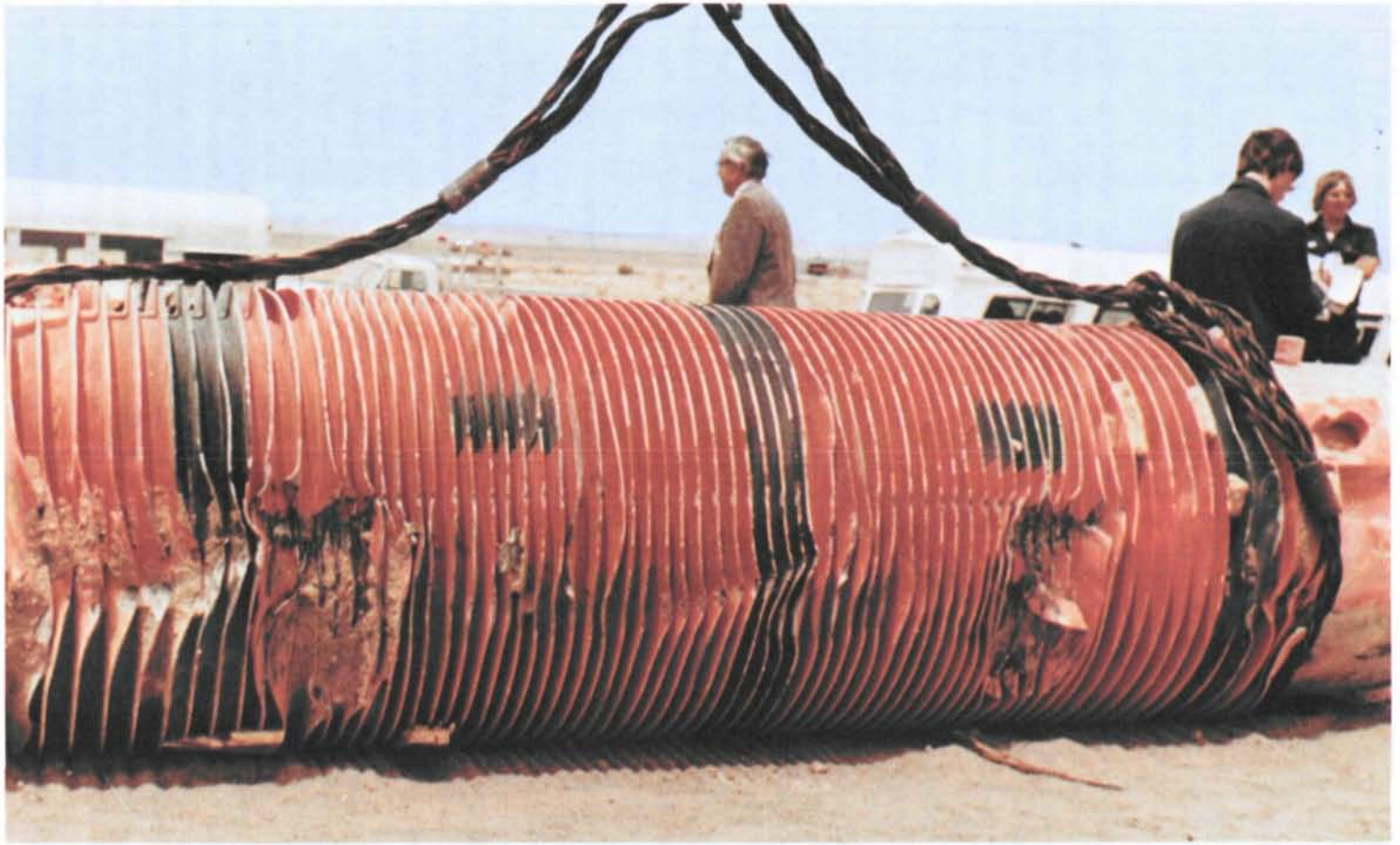
Figure 3. Fuel casks emerged from the crash tests with some exterior damage but intact. This cask was subjected to a full-scale vehicle test at 81.5 miles per hour. (Photo: Sandia Laboratories).
