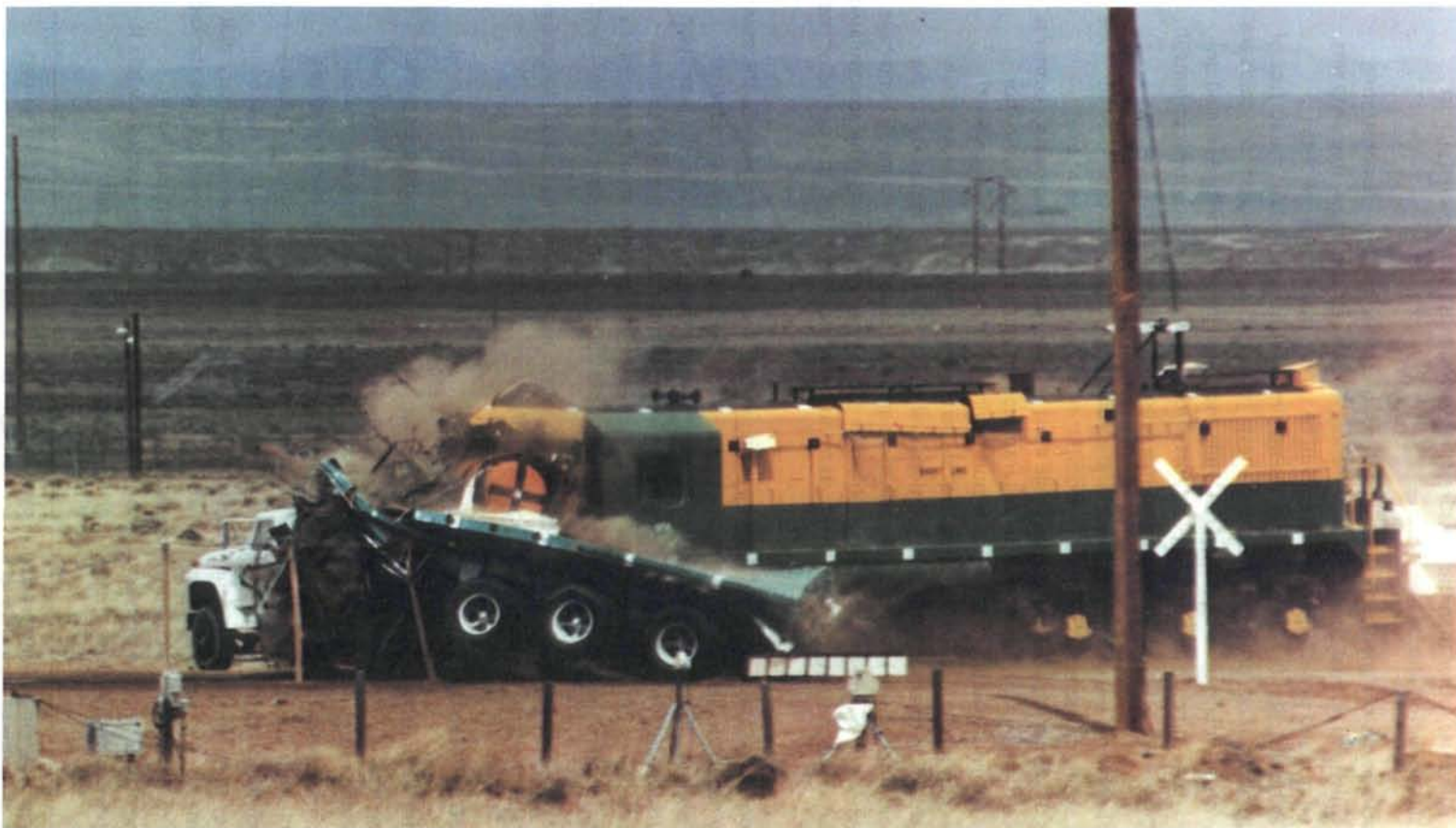
Figure 1. Spent fuel shipping casks have been subjected to a series of crash tests at Sandia Laboratories in the USA. In this full-scale vehicle test, a railway locomotive, accelerated to 81.5 miles per hour by rocket sled, was allowed to crash into a transporter loaded with a fuel cask (red object). (Photo: Sandia Laboratories).
