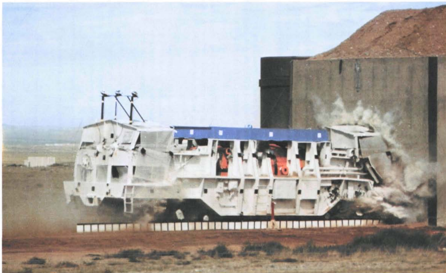
Figure 2. In another full-scale vehicle test, a railway wagon loaded with a fuel cask was crashed into this concrete wall at 81 miles per hour. (Photo: Sandia Laboratories).
