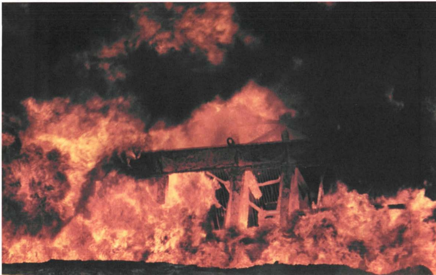
31 Figure 4. Rail wagon with a fuel cask undergoing a fire test. (Photo: Sandia Laboratories).
