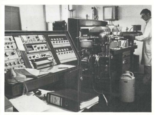
Single-stage surface ionization mass spectrometer (AVCO-type) requires 0.1 to 1  $\mu$ g samples of plutonium or 1 to 10  $\mu$ g of uranium.
