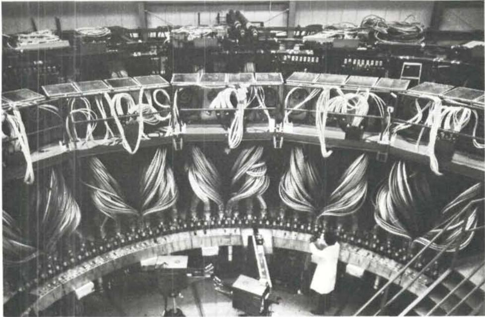
Scyllac, the toroidal theta-pinch experiment at the Los Alamos Scientific Laboratory, New Mexico, USA. The quartz discharge chamber is contained in the circular aluminium ring, with the many cables carrying the current required to energize the heating and confining magnetic fields. Photo: Los Alamos Scientific Lab. (photo 1)
