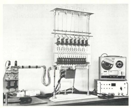
Automated radiochemical separator for the determination of cadmium, chromium, copper, molybdenum and zinc by neutron activation analysis. The samples, in a suitably oxidised form, are introduced into the separator in a dilute sulphuric acid medium. The radionuclides of interest are separated into three chemical fractions suitable for subsequent measurement with a NaI(TI) or Ge(Li) detector. Two samples are processed concurrently in about 30 minutes – UKEA Aldermaston
