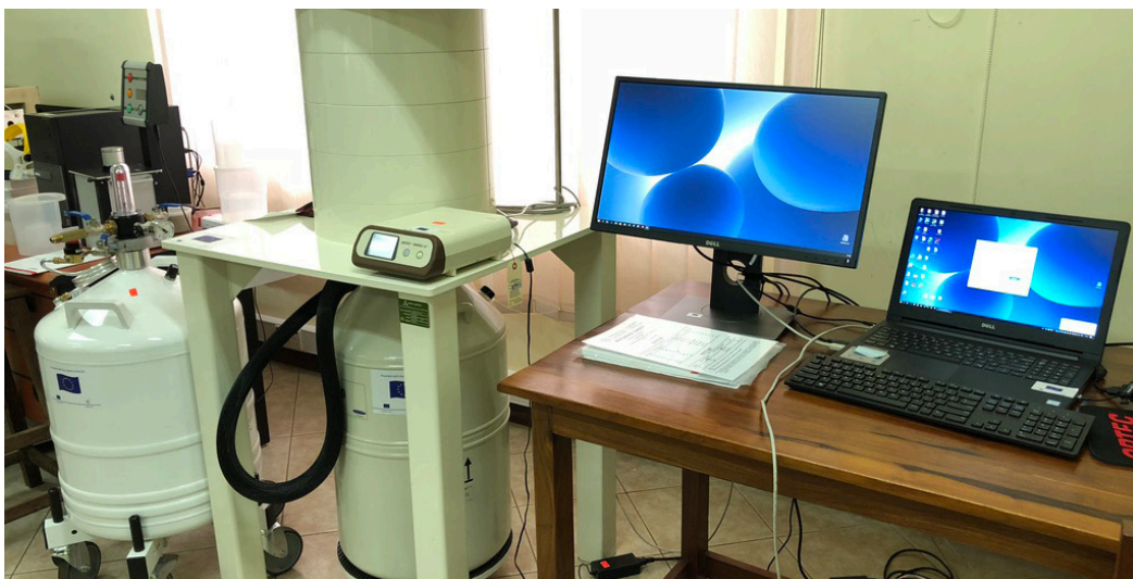
The uranium laboratory equipment includes a gamma spectrometry system, which will help authorities conduct a proper assessment for uranium found in the country.
