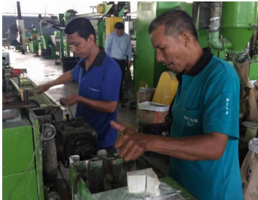
Cables such as these produced at Wonderful Ebeam Cable will be used in the engine compartment of cars. They are made heat resistant and fire retardant using irradiation.
