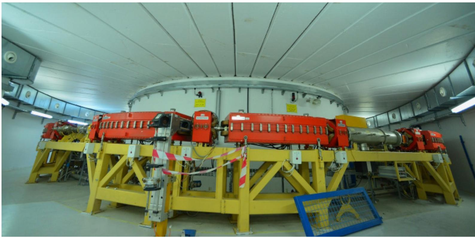
**3** This is the inner storage ring of the facility, where electrons start to circulate to build up the required energy of 2.5 GeV. The inner storage ring, or booster, with deflection and focused magnets, will enable the electron beams to circulate as they accelerate. The precise beams of light produced include microwave, infrared, visible, ultraviolet, X-ray and gamma-ray light.
