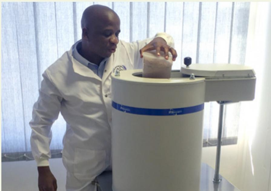
**A gamma spectrometer donated by the IAEA is used to measure naturally occurring radiation in Botswana.**
