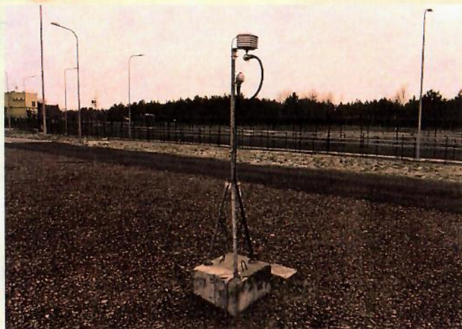
Radiation monitoring sensor at ISF-2
