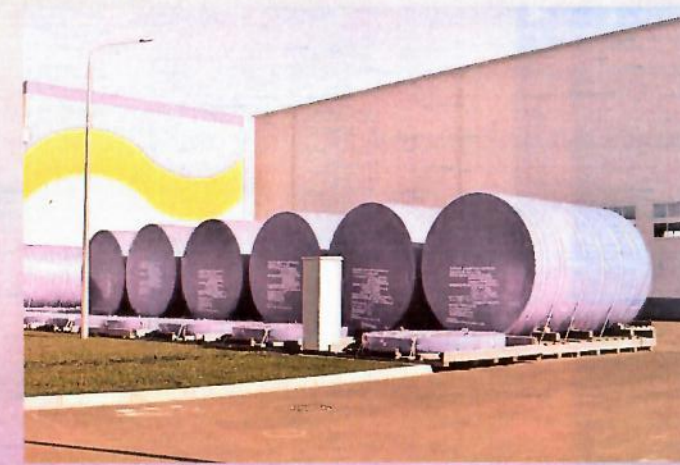
Casks for transportation of liquid radioactive wastes
