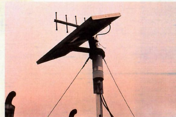
Autonomous radiation monitoring sensor "Rados"
