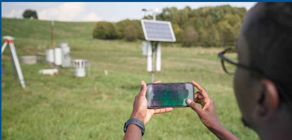
The cosmic ray neutron sensor seen in the background sends real time soil moisture content data to the phone in the foreground. (Photo: IAEA)
