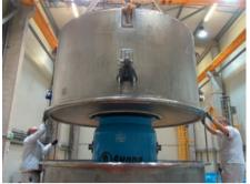
FIG. C.5. Tightening the bolts on special transport packages carrying spent HEU fuel from Viet Nam's Dalat Nuclear Research Institute to the Russian Federation (left). Placing a protective overpack on a transport cask containing spent HEU fuel from the BRR in Hungary (right). This overpack was designed to permit air transport.
