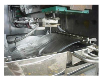
FIG. F.1. Treatment of wastewater using an electron beam accelerator (courtesy of EB Tech).
