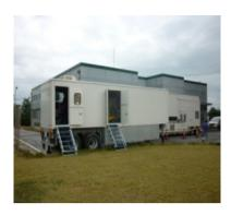
FIG. F.2. A mobile electron beam accelerator installed in sewage treatment plant (courtesy of KAERI).
