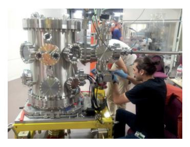
FIG. C.2. Assembly of the UHVC end station.
