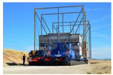
FIG. B.4. The ITER site as of September 2013 (left). The 800 t trailer with remote controlled vehicle, replicating the weight and dimensions of the largest ITER loads (10 m tall, 33 m long and 9 m wide), travelled at an average speed of 5 km/h for four consecutive nights to test the 104 km long 'special itinerary' (right) (courtesy of ITER).
