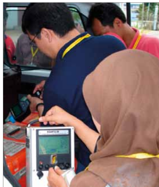
Participants in a training course learn how to use handheld detection equipment like radiation isotope identifiers, that with built-in spectrometers, can determine what type of radioactive material is present.
