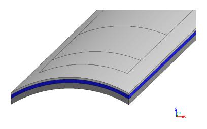
7 MeV Electrons on aTantalum, Water, Steel Sandwich
