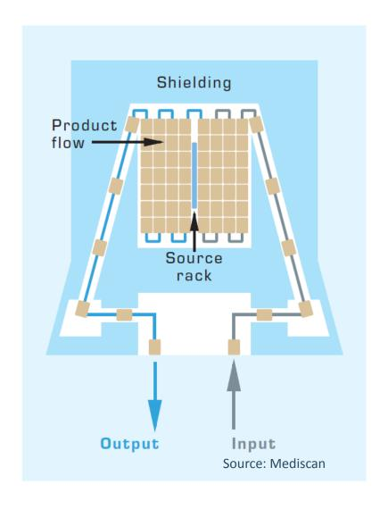
Reliable & Proven: Co-60 Isotope Decay High Troughput Good Penetration
