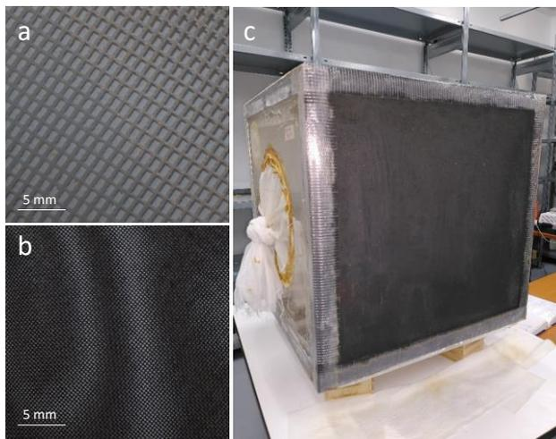
*Figure 2. Structure of the oviposition panel. (a) Internal and (b) External mesh nets constituting the wax panel; (c) The mesh nets are fixed to the holding cage frame using a strong adhesive tape.*
