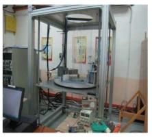
Radiation Source - Cs-137 Detector: Nal(Tl) - 2" x 2" Detector Collimator - 2 mm Programming - Expectation-Maximisation (EM) and Alternating-Maximisation (AM) algorithms written in Visual-Fortran programming language
