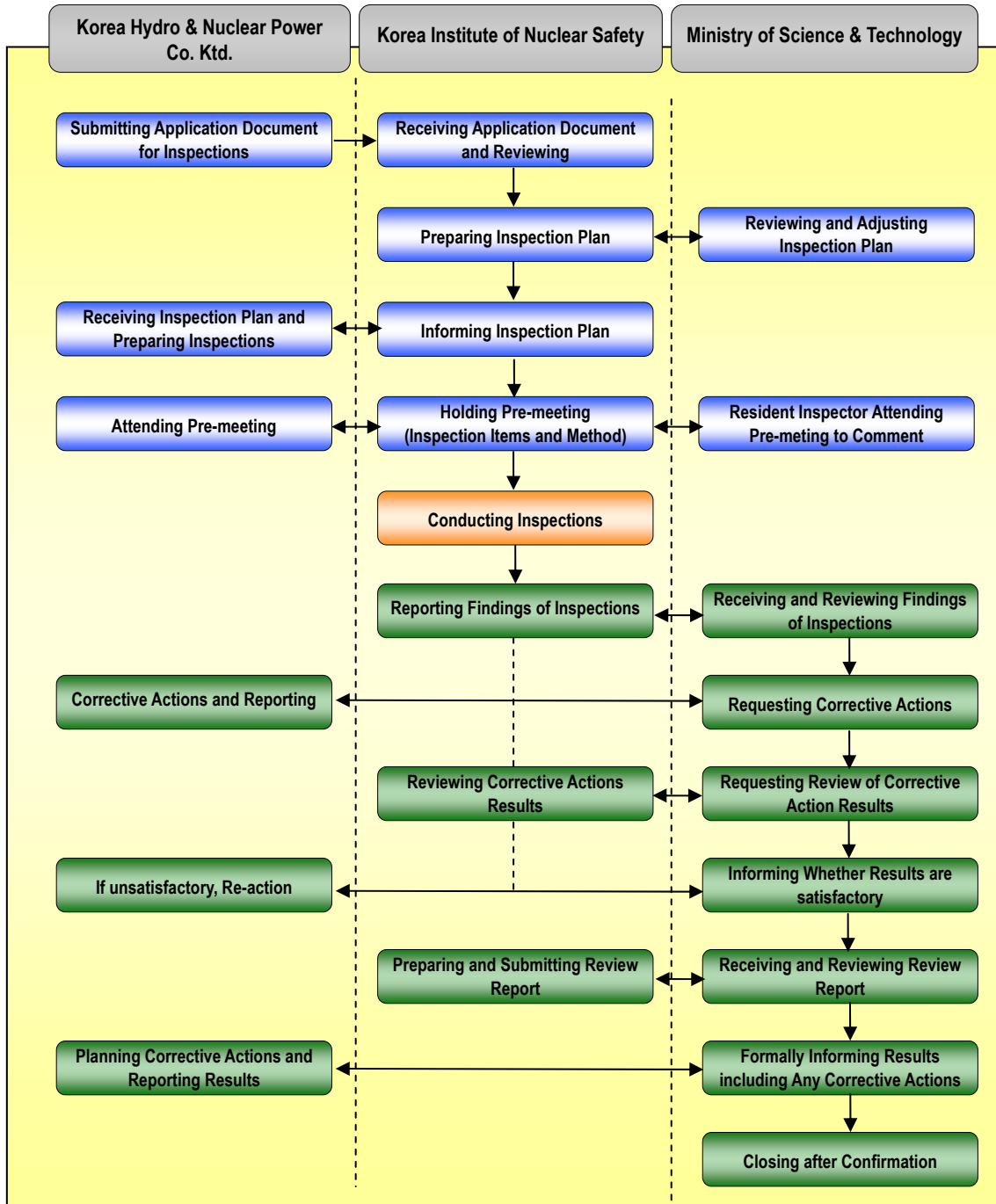
Figure II.2-5 Regulatory Inspection Process for Nuclear Installations
