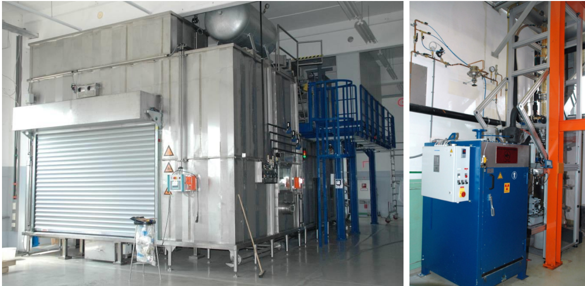
Figure 6: Drum drying system for up to 32 drums (left) and in-drum dryer for single drums (right), © NES
