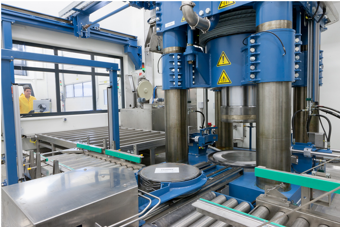
Figure 3: Supercompactor with parts of handling system, © NES
