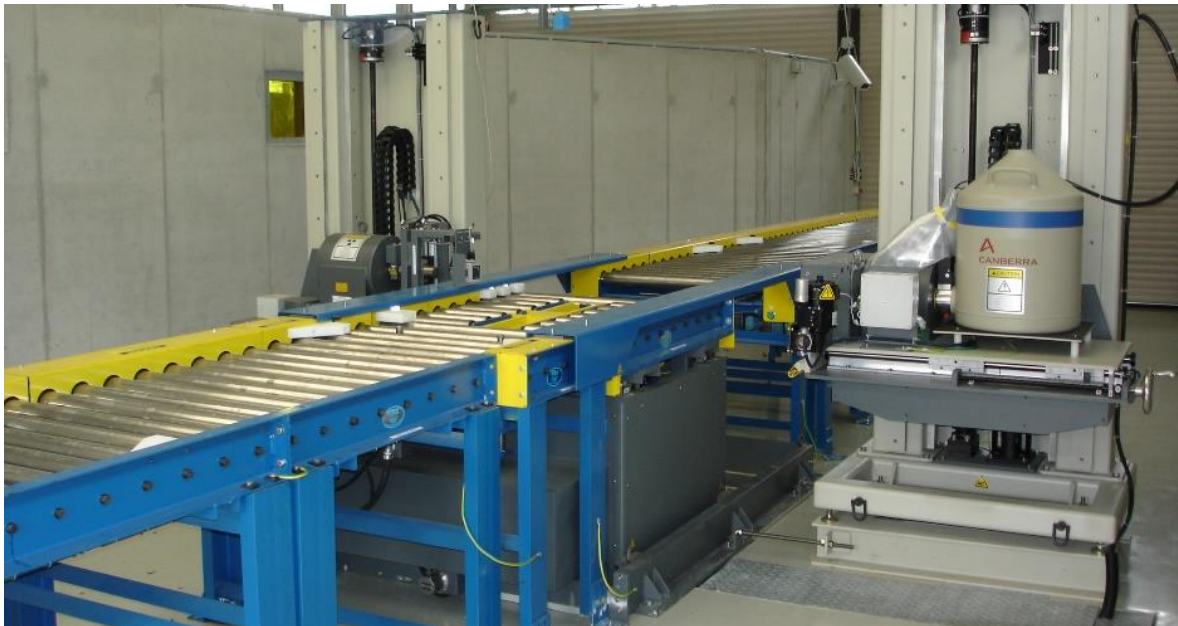
Figure 8: Waste Assay System in the measuring facility at Seibersdorf, © NES
