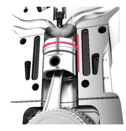
Surface of component irradiated by ions (protons or deuterons) in cyclotron
