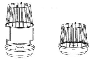
**CBDT** (Closed Bottom Dry Trap) - The dry trap body was a fluorescent green painted plastic she hat formed a 15 cm long, 9 cm diameter, cylindrical container having three 2 cm diameter holes 1 neet access. The bottom and the top of the trap consisted of two removable plastic petri dishes. T raps also contained a small toxicant square consisting of methomyl<sup>®</sup> + sugar to kill attracted flies.
