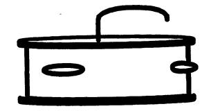
**BDT** (Open Bottom Dry Trap) - The body of this dry trap was a green plastic sheet that formed 5 cm long, 9 cm diameter, cylindrical container having three 2 cm diameter holes for insect acces he top of the trap was made from a plastic petri dish. A yellow sticky paper insert with a pre-applie dhesive was used to retain attracted flies.
