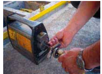
Typical iridium-192 shielding device. Photo: Chilean Nuclear Energy Commission
