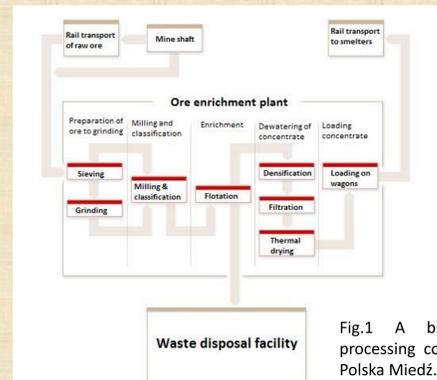
Fig.1 A block diagram of processing copper ore in KGHM Polska Miedz. Source: kghm.com
