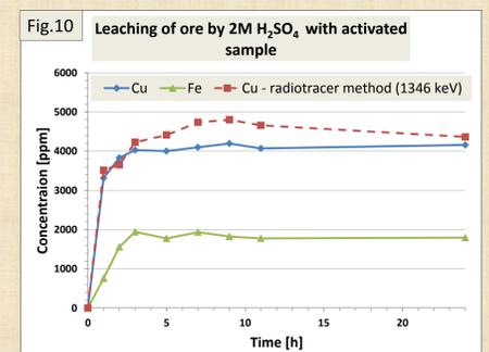
Figs 9-10 Exemplary results of leaching process using radiotracers
