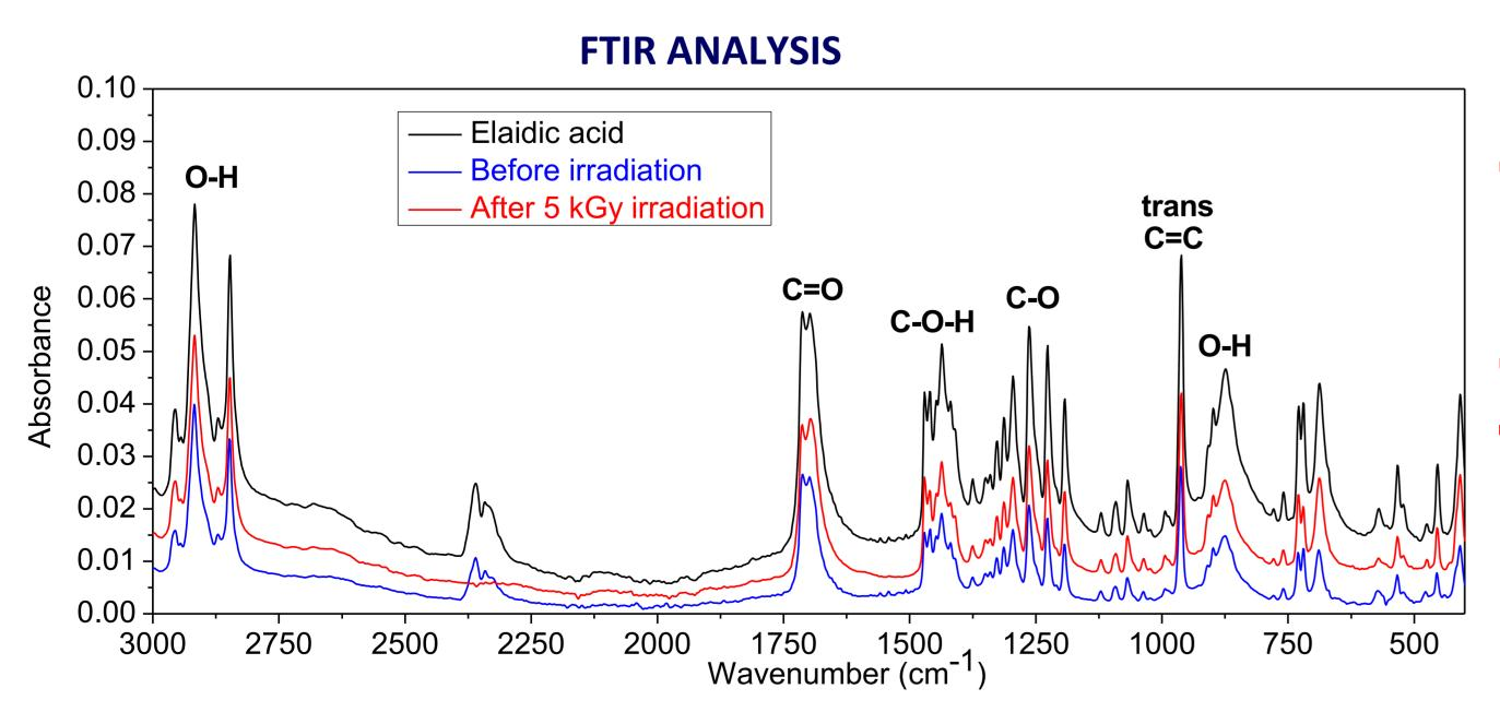
• FTIR spectra obtained on samples with a EA surface film non-irradiated and irradiated both showed the
