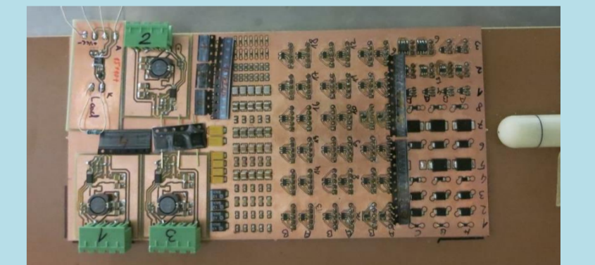
Electronic devices for satellite power supply mounted on PCB (Printed Circuit Board) with ionizing chamber on the right.
