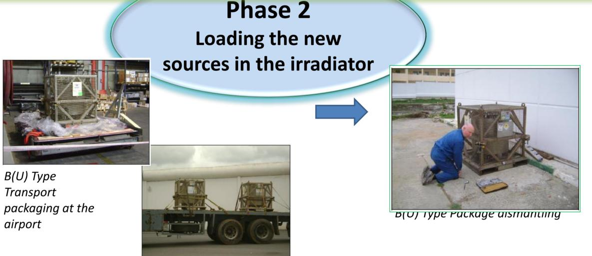
A smear test on the external surface and a leak test on the content done on both packages to prove that neither external contamination nor leakage of the sources occurred. Then the temporary pool will be rechecked, filled with water. The water level and quality will be maintained precisely. one of the supplier containers will be lowered into the pool.
