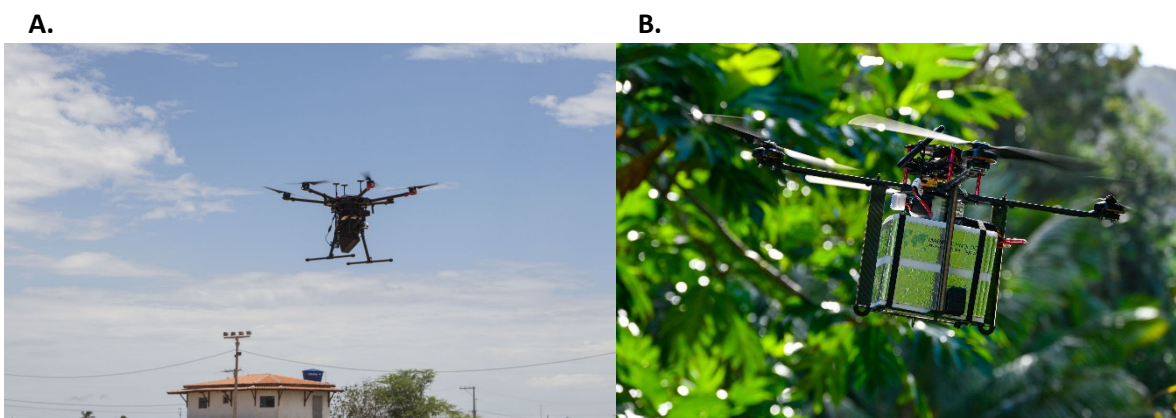
Figure 10. (A) Aerial releases of sterile male Aedes aegypti using a DJI Matrice 600 pro drone in Brazil (Photo WeRobotics) and (B) a custom-made drone in La Reunion island (Photo Pierre Marchal).
