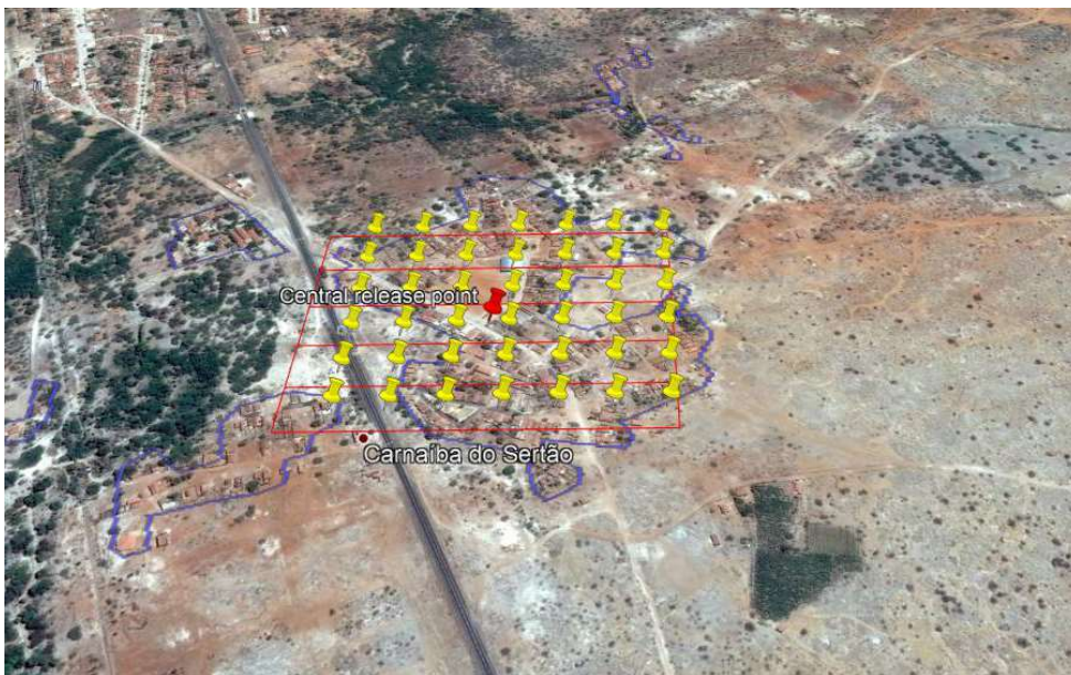
Figure 8. Release area of 20 ha in Carnaíba do Sertão. The red point is the central release point, the red lines are the release lines with a swath of 80m and the yellow points are the monitoring stations.
