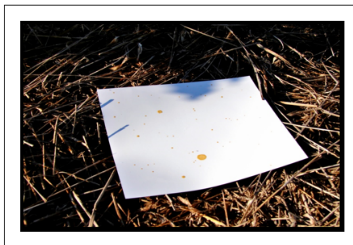
Figure 4.7. Kromekote cards (30 x 30 cm) showing the droplets of GF-120 after application of insecticide-bait by helicopter (Moscamed Programme, Guatemala).
