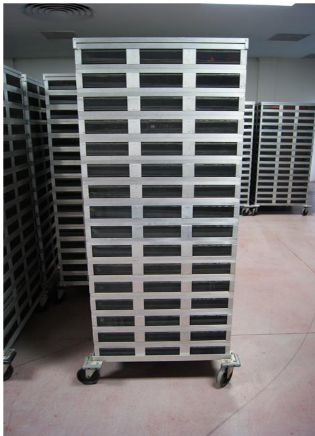
Figure 5.4 Mexico towers used to emerge and hold sterile flies. (©FAO/Programa Moscamed Mexico, Guatemala, USA)
