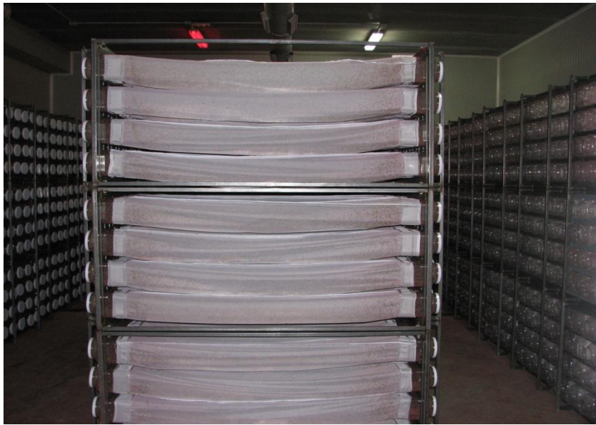
Figure 5.2 Fabric Sleeve cage, used to emerge and hold sterile flies. (©FAO/Programa Moscamed Valencia Spain)
