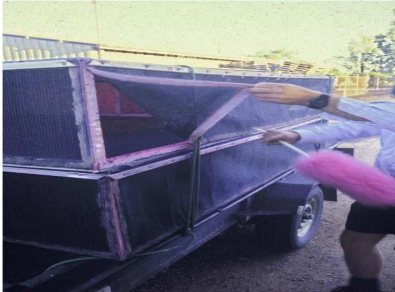
Figure 8.3 Two large mesh cages on a trailer. The sides are held with Velcro (i.e. material which has two sides, sticky hook side and a fur side – it can be pulled apart and pushed together to make a seal) and can be easily pulled open to release adult flies. Cages are transported in utility vehicles or trailers because of their size. This method usually releases large numbers of flies in a small number of confined release points. (©FAO/ Queensland Fruit Fly Program Australia)
