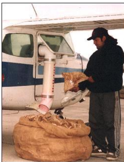
Figure 7.1 Typical chute used in aircraft for paper bag aerial release. (©FAO/Programa Moscamed Mexico, Guatemala, USA)
