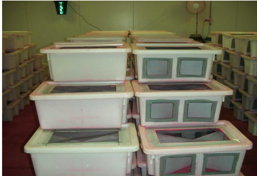
Figure 8.2 PARC boxes with and without ventilation in the sides. The internal divider for additional standing space can also be seen. Pink pupae can be seen in the bottom of boxes and emergence has not started. Boxes are stacked five high and room ventilation must ensure that waste gases do not accumulate in the boxes. (©FAO/ Queensland Fruit Fly Program Australia)
