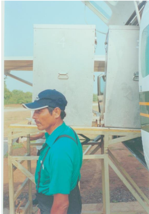
Figure 7.3 Release machine with a capacity of 10 million sterile flies per load. (©FAO/Programa Moscamed Mexico, Guatemala, USA)
