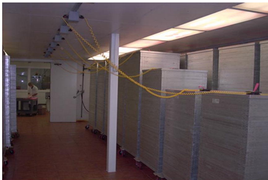
Figure 5.3 Worley Tower's used to emerge and hold sterile flies. (©FAO/USDA Mission Texas)
