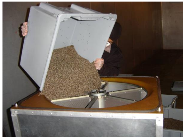
Figure 7.4 Double box release machine (DBRM). Shickel Corporation. (©FAO/Shickel Corporation)
