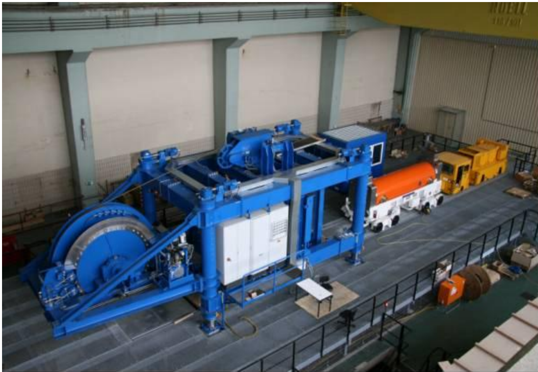
Figure D-7: Test stand for further development of the canister storage in boreholes
