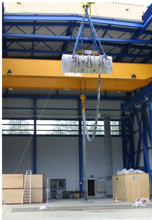
Figure G-1: Drop test of a transport and storage cask for vitrified waste, cooled down to minus 40°C, at the test facility of the BAM within the framework of an approval procedure under traffic law (Copyright: BAM)
