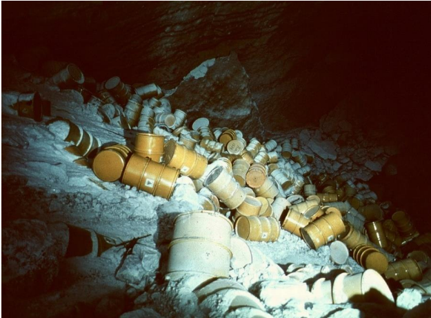
Figure D-10: Asse II mine (top left: waste packages dumped into an emplacement chamber (no longer accessible today) (Copyright: BfS), top right: view into emplacement chamber 7/750, bottom left: main collecting point for the uncontaminated solution on the 658 m level, bottom right: vibroseis vehicle during a 3D seismic measurement (Copyright: BGE)).
