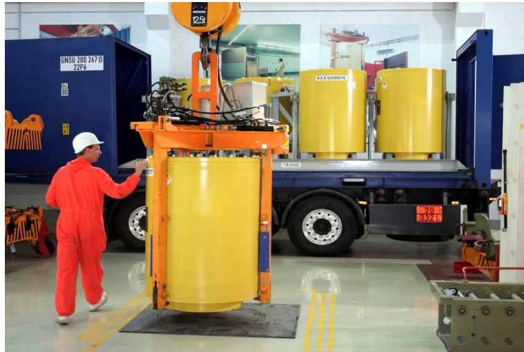
Figure F-2: Wipe test for product control on a MOSAIK container (Copyright: GNS)
