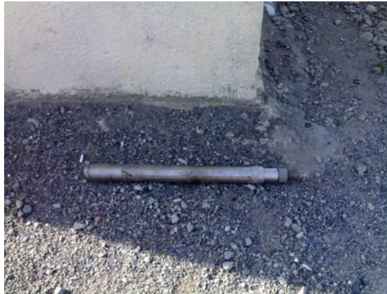
Fig.35 Plutonium/beryllium source found in the scrap metal shipment at the “Red Bridge on the Georgia-Azerbaijan border
