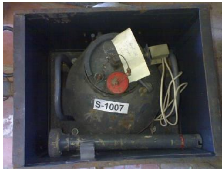
Fig. 39 Military container with one 10^{11}\text{Bq} activity ^{137}\text{Cs} source
