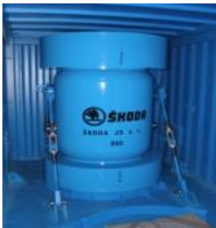
Fig. 11 ŠKODA VPVR/M container for transport of HEU from “Breeder-1”
