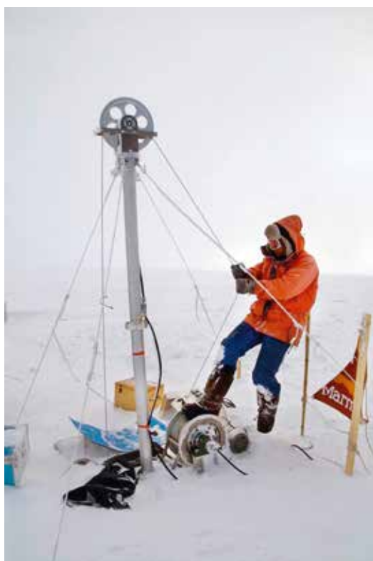
FIG. 2. Ice coring (up to a depth of 181.8 m) from the glacier at Elbrus Mountain, Russian Federation, for investigation of the palaeoclimate isotope record.
