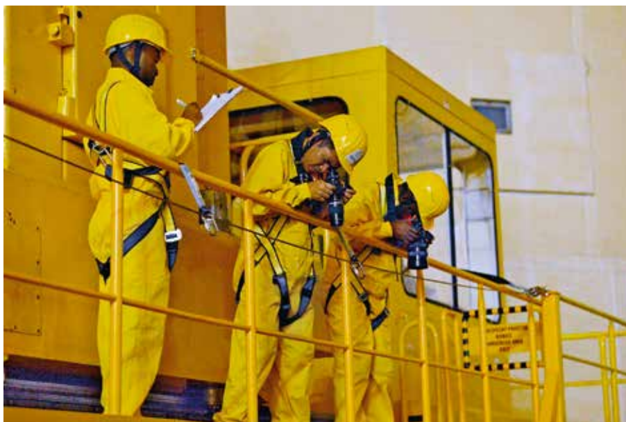
FIG. 3. Agency inspectors use non-destructive assay devices to verify spent fuel assemblies during a training exercise at Dukovany nuclear power plant in the Czech Republic in June.
