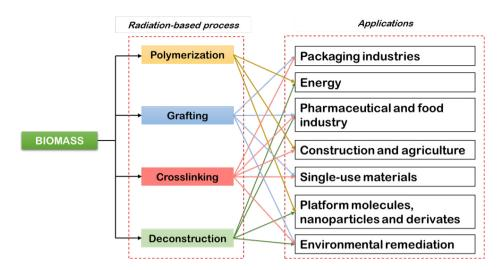
FIG. K.9. Overview of the use of radiation technologies to convert biomass into value added end products. (Graphic: IAEA)
