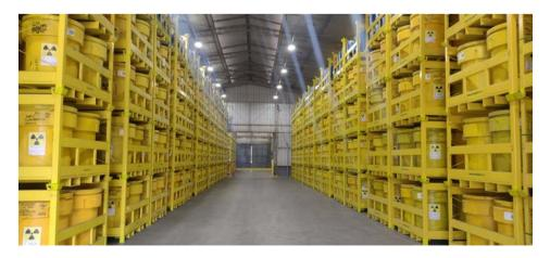
FIG. C.1. Storage facility for NORM waste from oil and gas operations. (Source: Petrobras)
