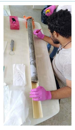
FIG. M.6. Sediment core preparation for radiochemistry analysis. (Photo: CIENAM, Federal University of Bahia, Brazil)
