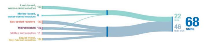
FIG. A.11. Breakdown of the 68 active designs in the Agency publication Small Modular Reactors: Advances in SMR Developments 2024. (Source: IAEA)
