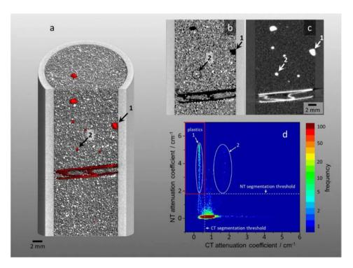
FIG. E.2. 3D rendered image combining neutron and X-ray tomography. The sub-volume containing a plastic particle is labelled '1'. (Source: J Soils Sediments 21, 1476 (2021)))
