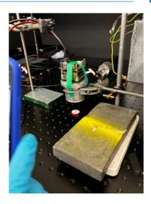
FIG. F.4. Compact scintillator-based gamma-ray neutron detector for terrestrial and space applications (ROSSPAD system) and experiment setup for testing purposes. (Source: Department of Technology Systems, University of Oslo, Norway)
