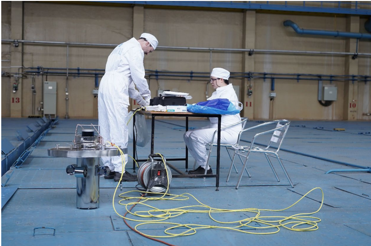
Safeguards staff deploying Robotized Cherenkov Viewing Device (RCVD) (Photo: IAEA)
