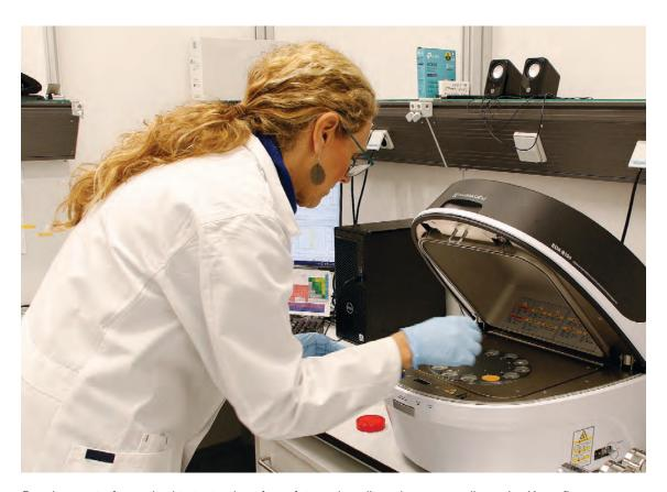
Development of a method to test spices for safety and quality using energy dispersive X-ray fluorescence spectrometry at the Joint FAO/IAEA Centre laboratories in Seibersdorf.
