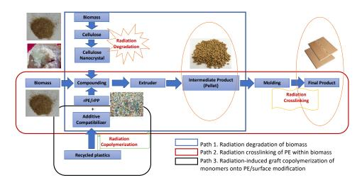
FIG. F-2. Scheme of the proposed production steps for reinforced wood–plastic composite with natural fibres and recycled plastics (recycled polyethylene and recycled polypropylene, rPE/rPP). (Image: National Nuclear Energy Agency of Indonesia)
