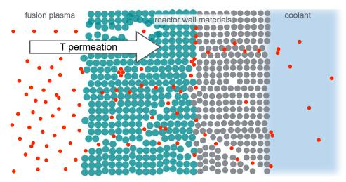
FIG. E-1. Schematic display of the tritium permeation process in a fusion reactor wall.
