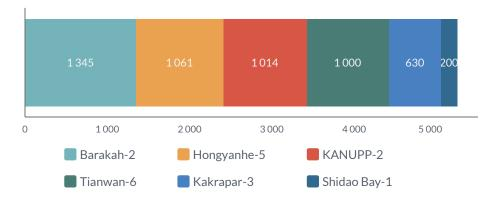
Hongyanhe-5 (1061 MW(e)) in China, KANUPP-2 (1017 MW(e)) in Pakistan, and Barakah-2 (1310 MW(e)) in the United Arab Emirates), one pressurized heavy water reactor (PHWR) (Kakrapar-3 (630 MW(e))) in India, as well as one high temperature gas cooled reactor (HTGR) (Shidao Bay-1 (200 MW(e))) in China (Figure A.3).
