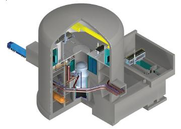
FIG. A-6. Canadian SCWR design — cutaway view of reactor building. (Image: Schulenberg and Leung, Canadian Nuclear Laboratories)
